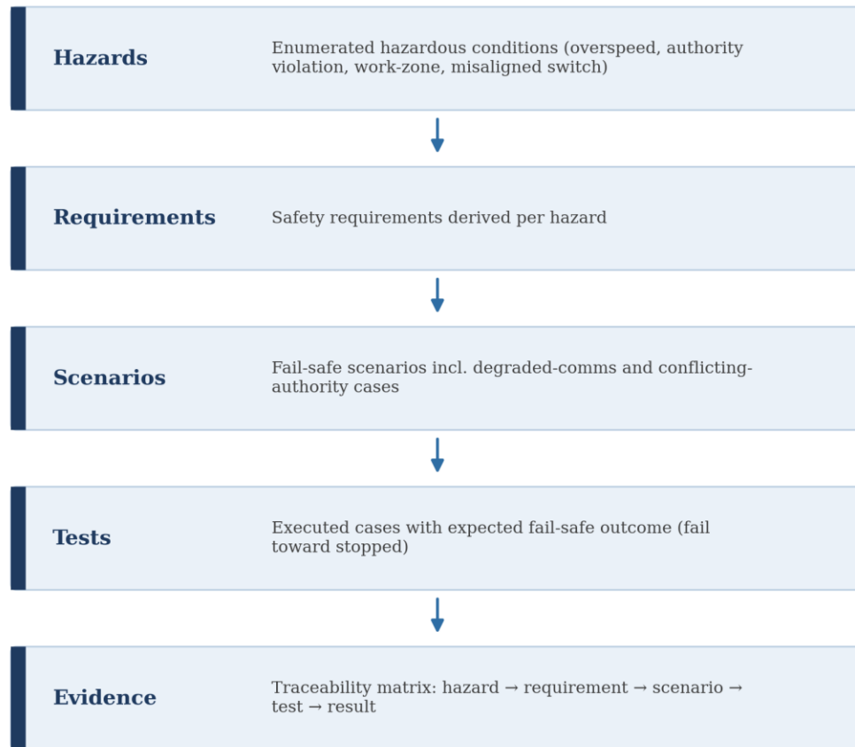
Figure 1. The traceability chain as a safety argument. The deliverable is not a green test run but a matrix in which any missing link is obvious.
